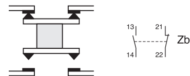
The 2 moving contacts are electrically separated
