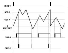
When count value rises above the level of the SET-1, OUT-1 is active and rises above level of the SET-2, OUT-2 is active. TOUT terms while selected HOLD, there is no outputs even to count value falls bottom level of SET values. Outputs will be reset when count value reaches zero (OFFSET), besides count value and outs will be reset when comes RESET.
