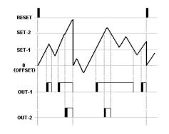
In this mode; when count value rises above the level of the SET-1, OUT-1 gives the out (so Relay-1 is ON). If TOUT-1 is selected (Time of Relay-1) HOLD, OUT-1 is active until count value falls bottom level of SET-1. When count value rises above the level of the SET-2, OUT-2 is give the out and If TOUT-2 is selected HOLD, OUT-2 is active until count value falls bottom level of SET-2. TOUT-1 and TOUT-2 are selected as term, OUT-1 and OUT-2 will active during this time.
