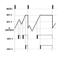
When count value rises above the level of the SeT-1, OUT-1 is active and rises above level of the SET-2, OUT-2 is active. So count value will be fixed. Even if encoder's pulse is at device without RESET, count value does not change but count value and outs will be reset.
