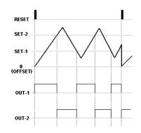
TOUT times should be selected as HOLD. OUT-1 is active until count value reaches the value of the SET-2 and OUT-2 is inactive when reaches. OUT-2 is active until count value reaches the value of the SET-1 and OUT-1 is inactive when reaches.
